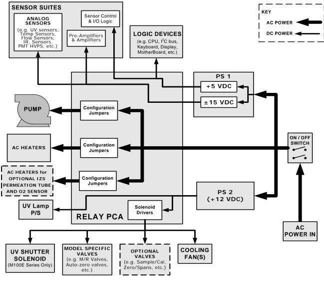
Figure 2-1: Power Distribution Block Diagram
